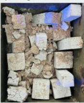
Figure 1: Thermal spalling at 800°C
