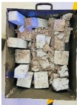
Figure 4: Thermal spalling at 800°C.
