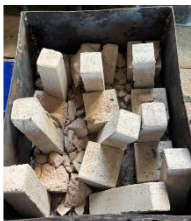
Figure 3: Explosive spalling at 600°C.
