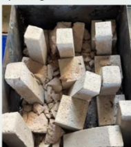
Figure 2: Explosive spalling at 600°C
